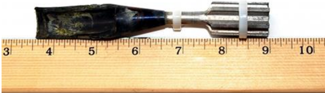
M101 spotting round showing depleted uranium in black.
